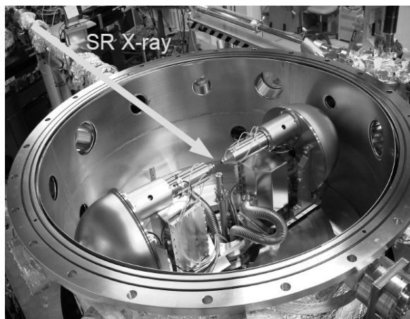
Fig. 2 Photograph of the angle resolved XPS machine. Two analyzers can rotate independently around the sample center in the UHV. On experiment, a manipulator is put on the center pillar.
